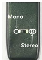
Whether you should use Mono or Stereo setting depends on your aircraft's avionics. Incorrect setting will result in communication being heard in only one side. For most general aviation aircraft the mono setting is required.
