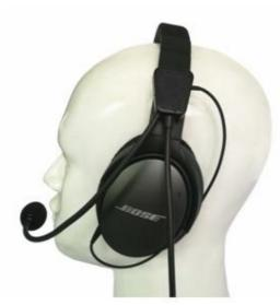
3. Using a cable tie secure the SM-1 tightly to your headphones (it is recommended to use 2 cable ties for improved stability and durability). Pull the cable ties as tight as possible then cut excess leaving around 1 cm protruding to make it easier to release and reuse in the future (extra cable ties and Velcro pads are supplied for future use as required).
