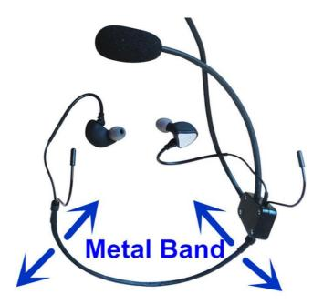
7. Ear loop adjustment - It is important that the ear loops feel comfortable when the headset is on. Hold the base of the loop and adjust the bracket openings to the desired shape for a comfortable, light fit. Please ensure you are not pulling the speaker wires
