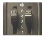
To adjust the comms volume move the sliders for the relevant ear.
