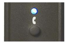
Press and hold the Bluetooth button for more than 1 second the SH30-75B will start to search for previously connected devices, if none can be found it stays in the search phase.
