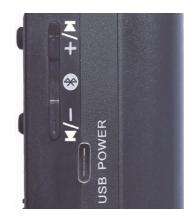
Press and hold the relevant button to adjust the Bluetooth volume (there is an audible tone when max or min is reached). Briefly tap the relevant button to skip tracks in the direction desired.
